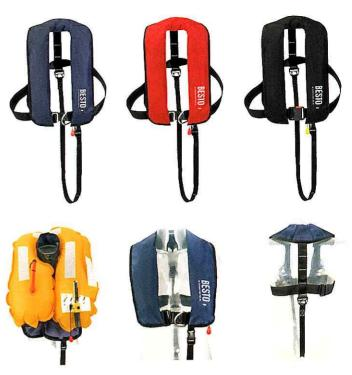
With its 3D design and soft outer cover, the Besto 165N has a perfect fit. The collar is firmly connected to the back and neck. Due the 3D fit it provides a safe and comfortable neck support. The jacket is fitted with a Crotch strap. This to make the jacket work better and gives an higher freeboard. The vest is finished with an edge bonding around. The vest has a buoyancy of 165N. The vest is available in several variations, automatic or manual, with or without harness and in various colors.
