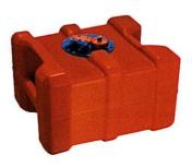
Tanks made in high density polithene plastic, suitable for acids and fuels, complete with standard inspection porthole with cap, vent, air-vent terminal 3/8", fuel pick-up and tank is ready to be used. The porthole is ready to take: a fuel gauge (mechanical or electric) elbow terminal of 1/4" for rubber hose as second fuel pick-up or diesel return, for fixed installation.
